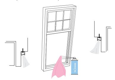
Carefully place the sash window back into the frame, ensuring that the window profiles fit into the frame profiles, and reconnect the balancing system.
