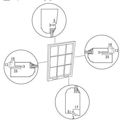
Cut the window strips on the left and right to the correct height, trim the O-profiles at the top (small) and bottom (large) to the correct width and press them into the rebates of the sash window.
