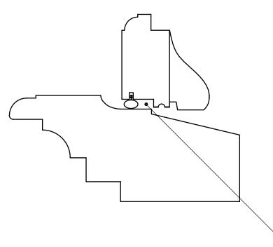
This position of the O-profile is also possible, but it creates a small gap between the O-profile and the strips on the sides.
