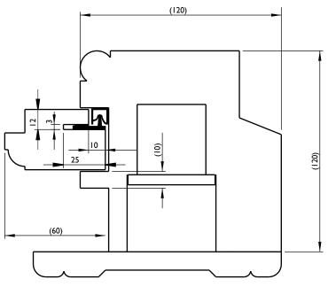
Coupled balancing systems with simultaneously or separately sash top and bottom sashes, as well as double-sash frames with shared weight in the central stile, can be easily implemented with VR Strips.
