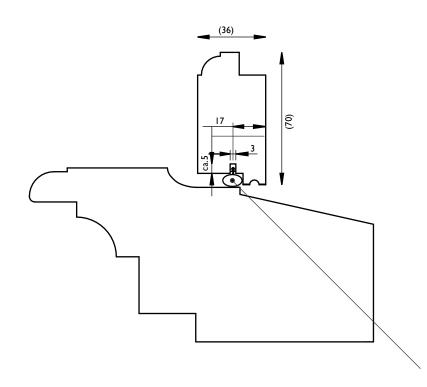
This position for the O-profile is ideal because it forms a closed frame with the strips on the sides.
