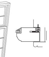
Reinstall the window into the frame, ensuring that the profiles interlock properly (see drawing). Approach the frame as straight as possible from the inside to ensure the profiles are immediately wellpositioned relative to each other. Stabilize the window securely before letting go. Reconnect the balancing system.
