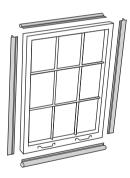
minimal adjustments to the sash window, VR Strips clamped into milled rebates
