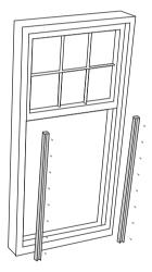
no adjustments to the window frame, only fastening the VR Strips into the rebate
