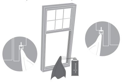
Carefully place the sash window back into the frame, ensuring that the window profiles fit into the frame profiles, and reconnect the balancing system.
